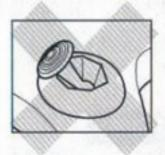
If the Control Stick is held at an angled position (as shown in the picture on the left) when the power is turned ON, this position will set as neutral. This will cause games using the Control Stick to operate incorrectly.
