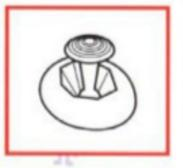
To reset the neutral position once the game has started, let go of the Control Stick so it can return to its center position (as shown in the picture on the left) then press START while holding down the L and R Buttons.
