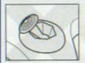
If the Control Stick is held at an angled position (as shown in the picture on the left) when the power is turned ON, this position will be set as neutral. This will cause games using the Control Stick to operate incorrectly.
